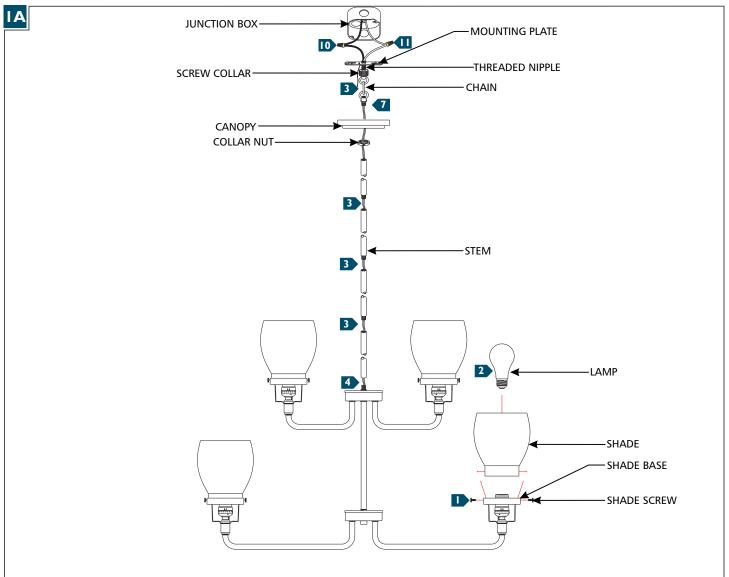
Align the holes on the shade with the holes on the shade base and secure it with the shade screws. Repeat for all shades.
